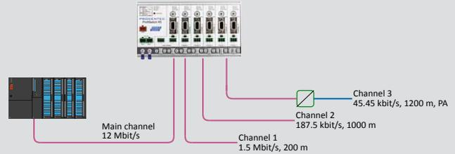
Example: one network, multiple baudrates, different cable lengths.
